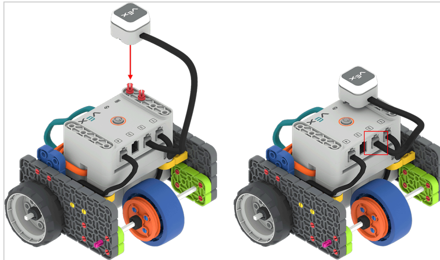
Add LED Bumper Sensor and Connect to Port 2
