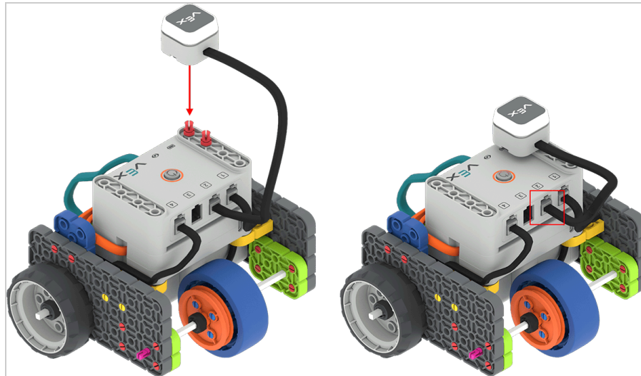
Attach LED Bumper to the Code Base, and connect to Port 2 on the Brain
